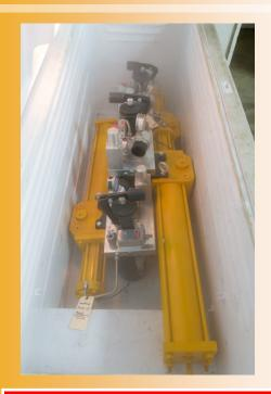
Each WCSCLP unit is frozen and tested for a MINIMUM of 24 HOURS to -22°F
