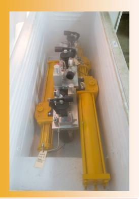
Each WCSCHP unit is frozen and tested for a MINIMUM of 24 HOURS to -22F
