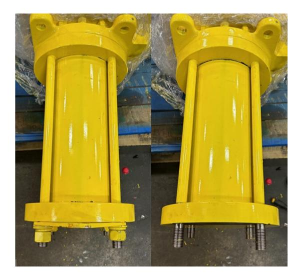
9.1.3 Remove the End plate and piston housing.
