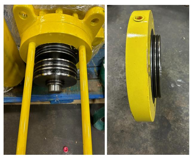
9.1.5 Reinstall piston housing, taking care to not cut of pinch any of the O-Rings. Reinstall cover plate and end nuts onto body screws and tighten evenly.
