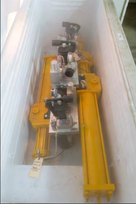
Each WCM Hydraulic Actuator Series Actuator is frozen and tested for a **MINIMUM of 24 HOURS**
