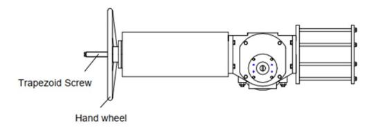
After manual operation, return to original position so to ensure auto-operation can be resumed. Avoid fully removing integral trapezoid screw, the valve open & close position will be influenced if the screw is positioned incorrectly.
